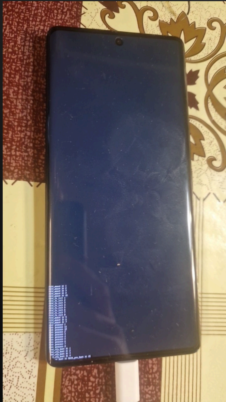
Framebuffer writes in LK bootloader
