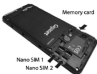
Slide the nano SIM card(s) and memory card into the designated slot. Do not apply force when inserting the SIM and memory card - the connector on the phone and other parts may be damaged.
