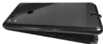
Use your fingernail to grip the notch at the bottom left corner and pull the back cover upward.
